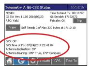
Adjust the YAGI antenna to the bearing and inclination.
