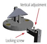
Fine tune horizontal and vertical alignment by adjusting screws until bubble moves to center ring in level. Replace barrel onto base, and close spring latches.
