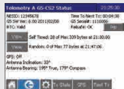
This screen will read 'GPS: Off'. This is normal as the station will only turn on the GPS while it is looking for a fix. Below this the antenna inclination and antenna bearing are listed.
