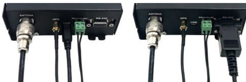
Figure 6: 6-DB with interface connections with USB cable (left) and RS-232 cable (right).
