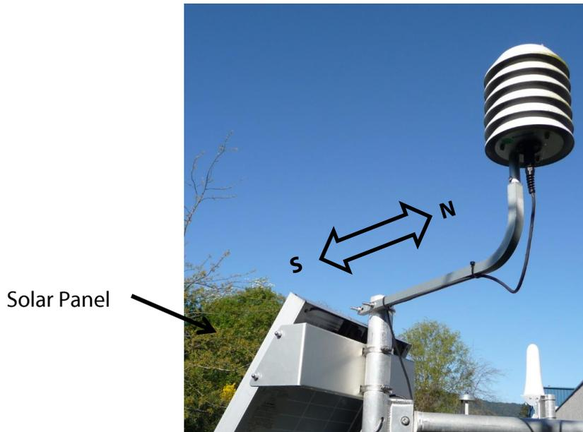
Figure 2-3: Support arm positioning (northern hemisphere)
