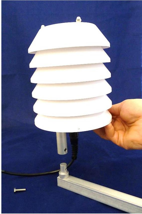
Figure 2-1: Attaching the assembly to the support arm
