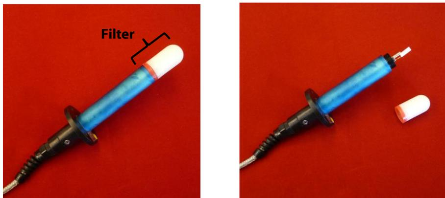
Figure 2-5: THS showing filter on and filter off
