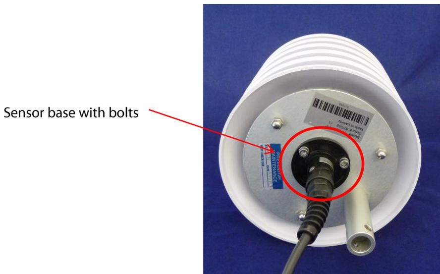
Figure 2-4: Sensor base showing bolts
