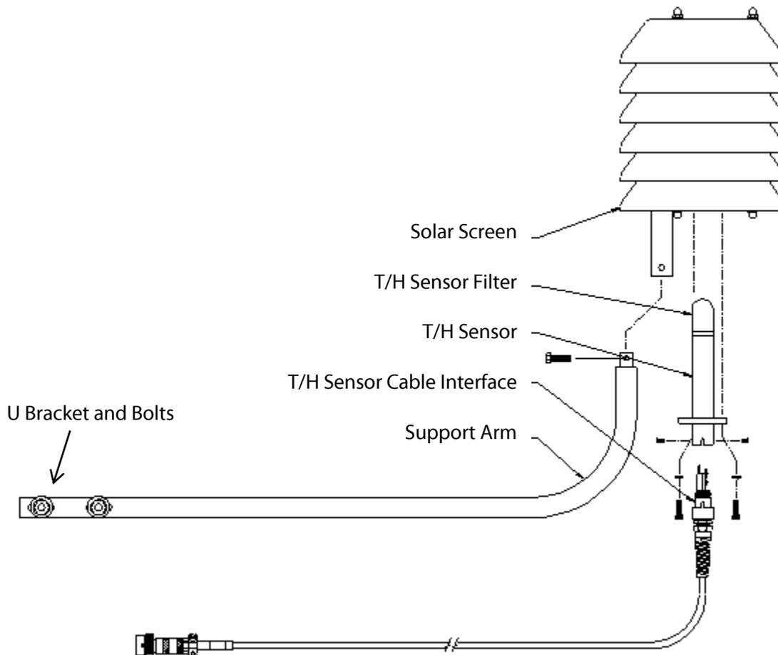
Figure 1-1: THS-3 Temperature and Humidity Sensor – Exploded View
